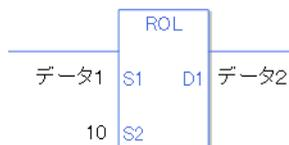
$$\{ \text{データ1} = 1 \text{ Step} \} + \{ 10 = 1 \text{ Step} \} + \{ \text{データ2} = 1 \text{ Step} \} + \{ 1 \text{ Step} \} = 4 \text{ Step}$$
