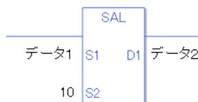
$$\{ \text{データ1} = 1 \text{ Step} \} + \{ 10 = 1 \text{ Step} \} + \{ \text{データ2} = 1 \text{ Step} \} + \{ 1 \text{ Step} \} = 4 \text{ Step}$$
