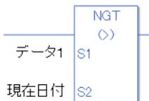
$$\{ \text{データ1} = 1 \text{ Step} \} + \{ \text{現在日付} = 1 \text{ Step} \} + \{ 1 \text{ Step} \} = 3 \text{ Step}$$
