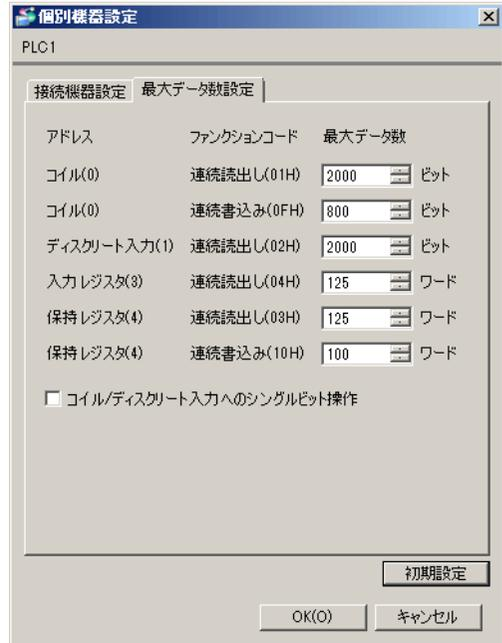
個別機器設定 dialog box (PLC1) showing the '最大データ数設定' tab. It contains a table with columns for 'アドレス', 'ファンクションコード', and '最大データ数'. The table lists various data points like coils and discrete inputs with their respective function codes and maximum data counts. Buttons for '初期設定', 'OK(O)', and 'キャンセル' are at the bottom.
